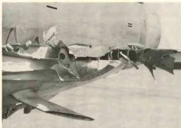
Releasing while rolling and pulling excessive Gs only serve to negate the bomb ejection velocity provided by the MER. This shows what a 750 pound bomb can do.
