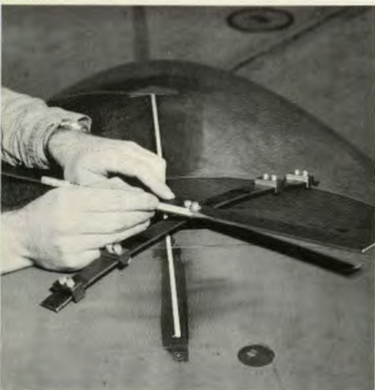
Locally devised yaw string jig. Actually it's a custom fitted "T" square fabricated in the 4th TFW machine shop. Pencil points out machined edge of the jig.
