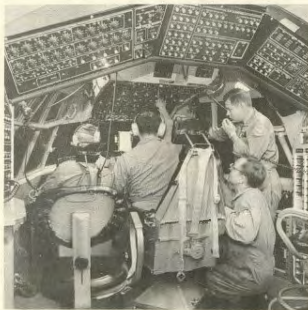
Thousands of ground hours are flown annually in C-130 simulators of 4442nd CCTW, Sewart AFB. Trainees learn to cope with many inflight hazards before their first actual flight. Instructor pilot and crew chief work with same aircrew through all flight training phases. This simulator flight is supervised by Capt. John R. Humm (standing) and SSgt. Alfred Blanche.
