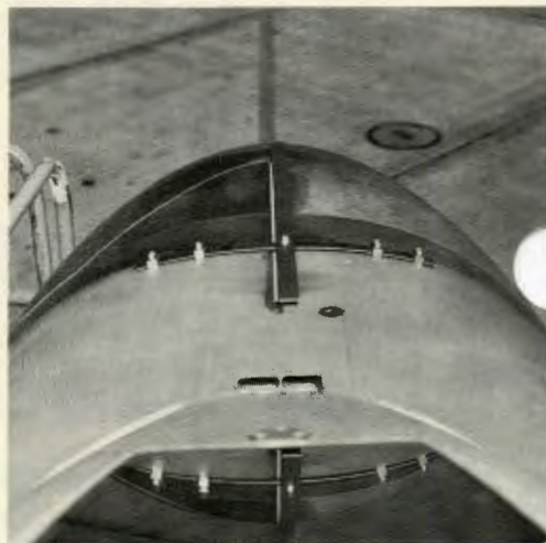
Run 1/16 inch reference line through the center screw of the rain removal access plate.
