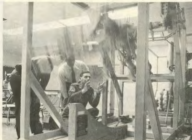
Aircrew trainees watch each component of C-130 nose gear. This mock-up swings gear through its full arc and is actuated by same hydraulic and control systems used by Hercules crews. The Sewart AFB ground school instructor is MSgt. Wayne Anderson, 304th FTD, and students are Capt. Xavier Garza (left) and Maj. Dan Dillon.
