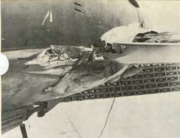
Thanks to the Thunderchief's railroad track-slab-spar, this aircraft made it home. Damage was caused by a pylon tank.
