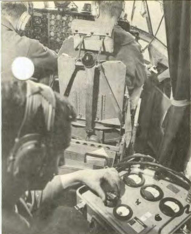
Keeping Herkys tuned for safe flight was a major contribution to the C-130's greatest operational year and lowest accident rate. Here, ground crewmen of 36th TAS, Langley AFB, use testing gear to check cockpit gages for proper indication of engine phase and RPM.
