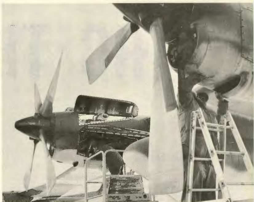
FOD is a constant hazard in keeping the Hercules humming. Engine intakes are checked by 37th TAS quality control inspectors, TSgt. John Horner (left) and SSgt. Lenard Catlett, at Langley AFB, Va.
